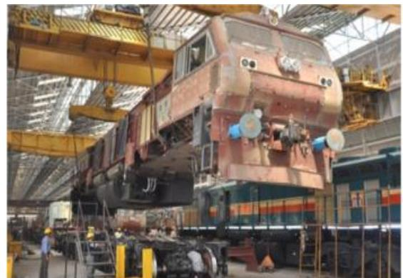
*Assembly of Diesel Locomotive*
