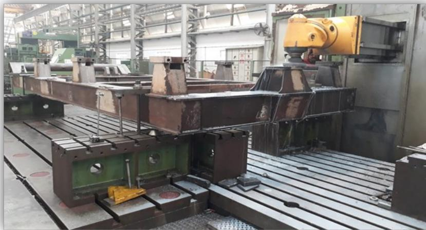
After complete fabrication stress relieving and shot blasting is being done for complete Bogie Frame. Final Bogie Frame is being machined in Heavy machine shop on CNC Horizontal Boring & Milling machine. After machining of Bogie frame assembly, set up and welding of small components is being done. After final inspection by Quality assurance department, bogie frame assembly is being undertaken for painting in Paint shop.
