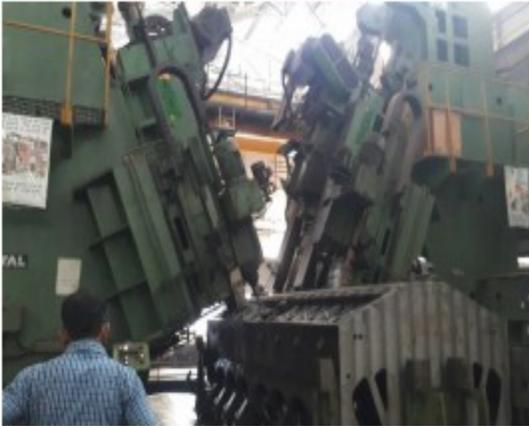
Angular boring or Liner boring of Crank case is done on this special purpose machine, which has two high precision angular boring bars at 45 degree on which different boring cartridge inserts are mounted. The machine is capable of boring and drilling to different sizes. The cartridge with inserts is mounted on boring bars to achieve evenly distributed cutting load during boring operation. This contributes to accuracy while machining.
