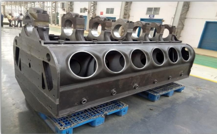
Prototype 12-Cylinder HHP Crankcase for Mozambique Railway
