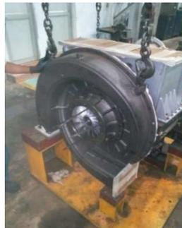
**2.2 Impeller Eye Clearance check in Hung position (2<sup>nd</sup> stage)**
